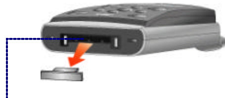
In-car Connector: Connecting hands free/car kit adapter and data manager cable. (Refer to page 68) * Always put rubber plug in this part to prevent contact from metal which causes power off. * When the power is off, remove the battery and insert it again and switch the power on.
