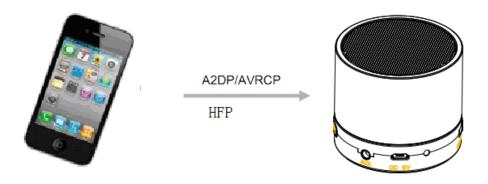
A. Slide the switch to "side, Blue LED flashes twice and 2 seconds later speaker will enter into Bluetooth pairing mode.
