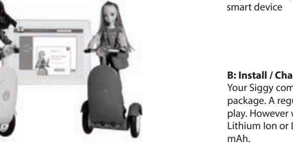
Siggy, is a fun app-controlled, self-balancing, inverted pendulum robot that is controlled by the SmartGurlz app - SugarCoded.
