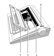
Setting Up Before you can use your typewriter, you must remove the packing materials from the print mechanism. This is essential to the proper functioning of your typewriter. Do not turn the unit on until you have prepared the typewriter for use. Follow the steps listed below using the typewriter diagram for reference. The numbers on the diagram correspond to those in the instructions. 1. Tilt the protective cover (1) toward you.
