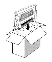
Place at least 2" of packing material in the bottom of the box for cushioning.
