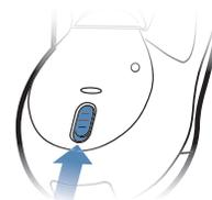
5 Insert the USB receiver into an available USB port on your computer.
