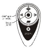
The RemotePoint Presenter Remote has four programmable buttons in addition to the laser pointer button and the ClickTrigger on the back.
