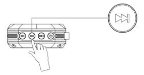
Quick Press to switch to next track.(Available only in Bluetooth) Press and hold it to turn up the volume.
