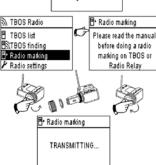
**6** If tagging has failed, the message "FAILURE CODE 1" will be displayed after a few seconds (1 indicating a radio error).
