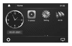
F-camera:Turn on the front camera. **Setup**: Shows the Settings interface. AV-In: Shows the AUX interface. Screen off: Turns off the screen, to reactivate the screen simply press any part of the screen.
