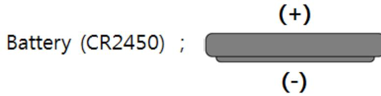
**Figure 15. Battery Directional**
