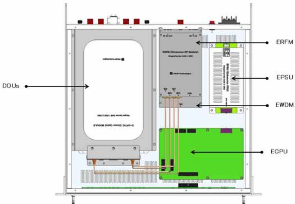
Figure 4.22 – OEU internal view
