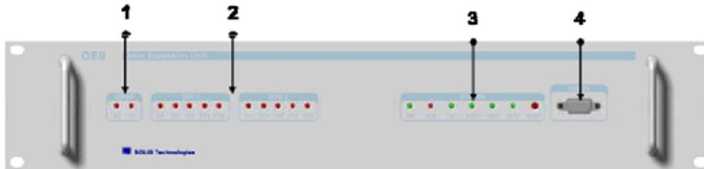
Figure 4.23 – OEU front panel Outer Look
