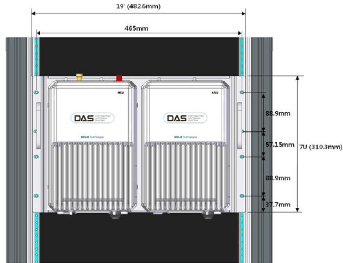
Figure 5.19 – ROU installation diagram for vertical rack
