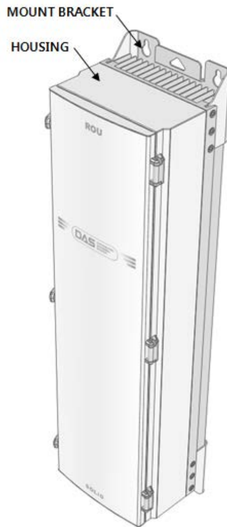
Figure 4.1 – Exterior of Remote Unit
