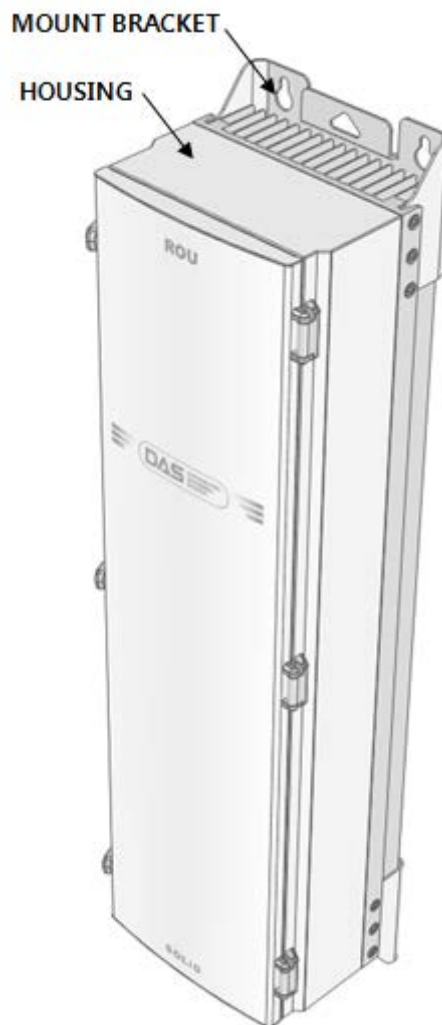
Figure 4.1 – Exterior of Remote Unit
