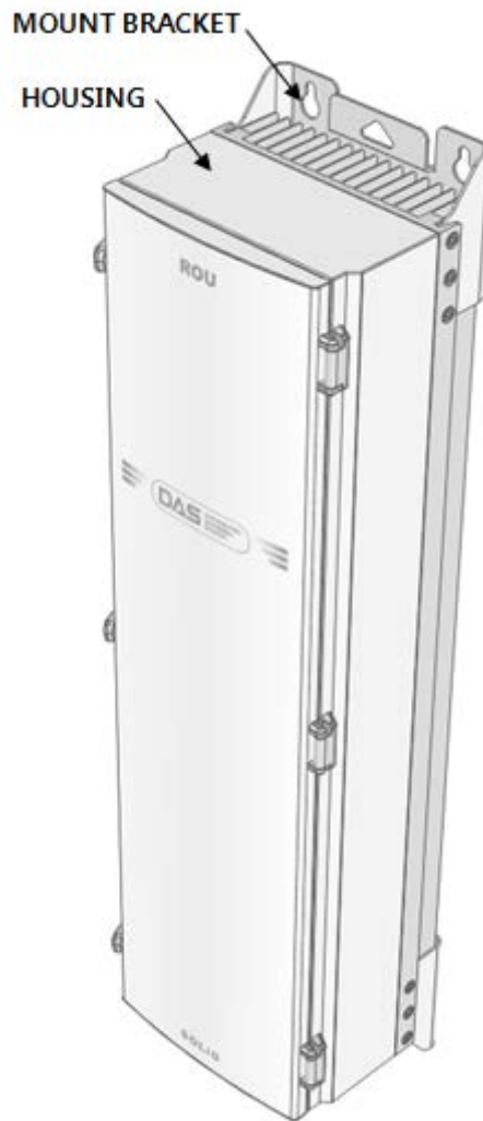
Figure 4.1 – Exterior of Remote Unit
