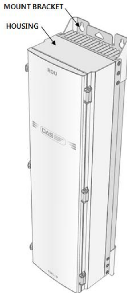
Figure 4.1 – Exterior of Remote Unit
