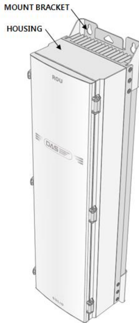
Figure 4.1 – Exterior of Remote Unit
