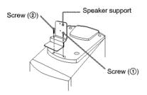
2 Insert the speaker support in the slot of the front speakers. Tighten two screws while threading the rear boards of the front speakers.
