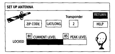
To determine the elevation and azimuth settings for the Satellite Antenna, select ZIP CODE or LAT/LONG.
