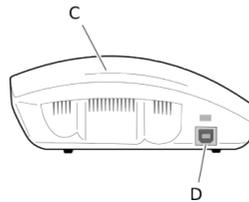
**C:** Status light. **D:** Power supply inlet (cable with the orange mark).
