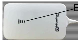
**E:** The array of blue LEDs is a locator.
