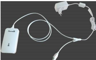
1 Power supply (European plug) with telemetry head
