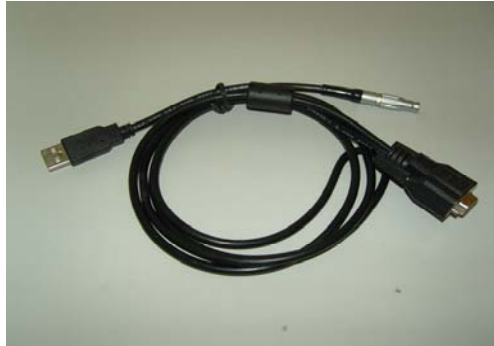
Figure 2-6 Data communication cable
