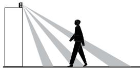
3.6 If mounted at a height of 8-9 ft above the floor, the detection range will be approximately 16 ft. with a  $110^{\circ} \pm 10^{\circ}$  view angle. If mounted at a lower height, the detection range may be decreased.
