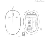
1) left button 2) right button 3) Wheel button (4) battery warehouse (5) receive
