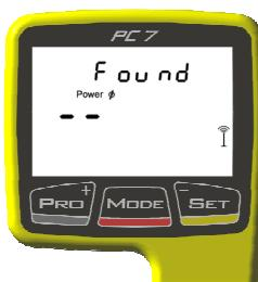
If a Sensor is found, the PC 7 will show "Found" in the Top line, alternating with the Sensor's Serial number.
