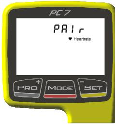
To pair another Sensor, press **MODE** once quickly to get back to the device selection Menu. Continue with pairing the Heartrate sensor and Speed sensor.
