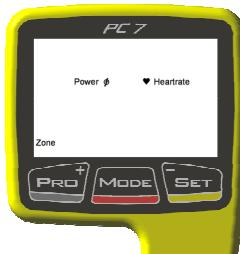
The fifth screen offers the possibility to choose the settings for training zones defined with heart rate (bpm) or power (watts). These can also be set through the SRM Windows Software.
