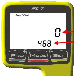
The first screen shows the Zero Offset Menu for the PowerMeter.
