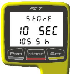
The fourth screen shows the setup menu for data storage. The storage interval can be set between 0.5 and 5.0 sec. By increasing or decreasing the storage interval, you will also increase or decrease the amount of memory available. For example, a storage interval of 1 second the memory will hold about 1054 hours, while a storage interval of 2 seconds will hold about 2108 hours.
