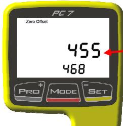
After the top number stabilizes, press **SET** to store the new **Zero Offset** of the PowerMeter.
