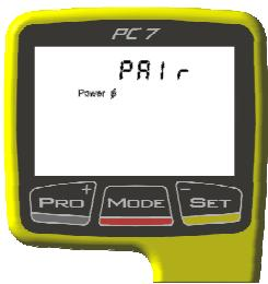
Hold **PRO+** for about 3 seconds to enter Sensor Pairing mode.
