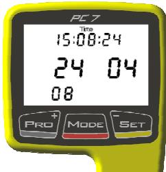
Hold **SET** for about 3 seconds to enter the Setup mode.
