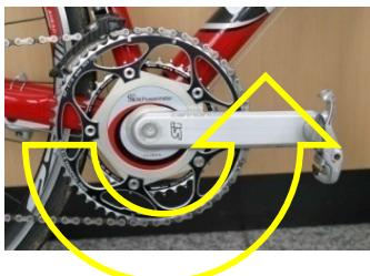
If the top number is zero, turn the PowerMeter on by pedaling backwards. Then, **let go of the crank and make sure nothing is touching it**.
