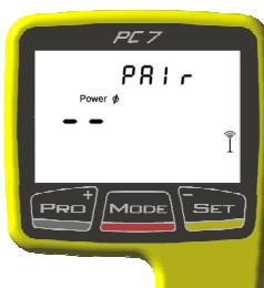
The Antenna symbol
