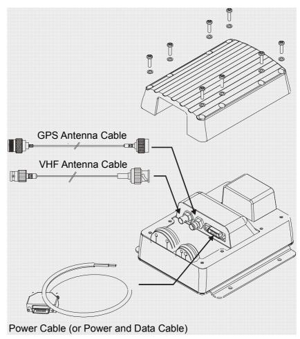
Replace the top of the transponder unit taking care to seat the cable grommets and the lid seal correctly. Do not over-tighten the fixing screws.
