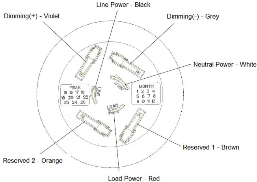
**Figure 4 - LCU NEMA 7-Pin Contact Interface**
