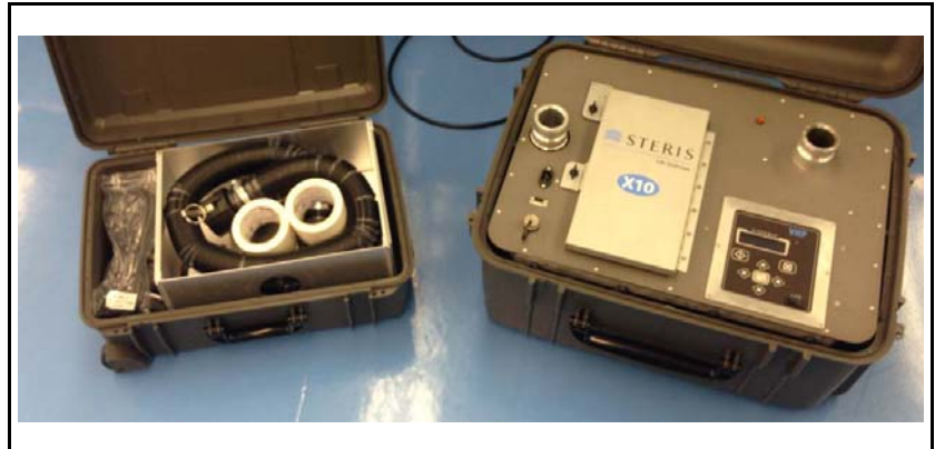
Figure 6-1. X10 Biodecontamination Unit
