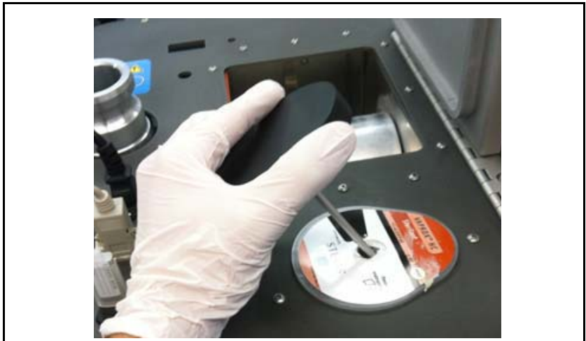
Figure 6-5. Carefully Insert Draw Tube (Typical)
