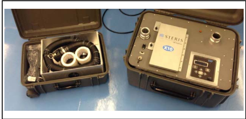
Figure 6-1. X10 Biodecontamination Unit
