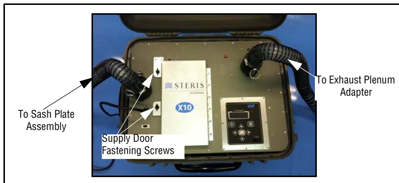
Figure 3-4. Connect Biodecontamination Unit to Enclosure
