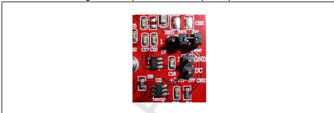
Figure 4. Jumper JP1 set in RF power position
