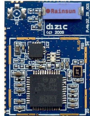
FRONT END WITH RF POWER LEVEL DETECTOR
