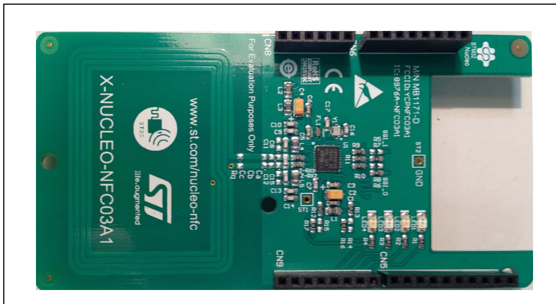
Figure 1: NFC card reader board based on CR95HF IC
