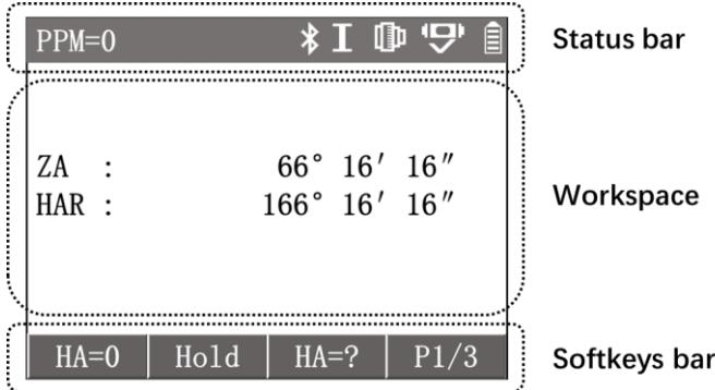
**Status bar:** Displays the current measurement status information icons under the measurement interface. Other interfaces indicate the name of the current interface or procedure, as well as necessary information icons.
