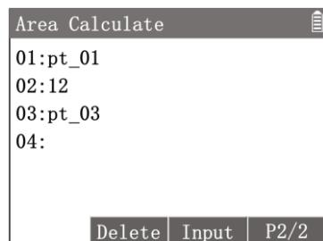
After getting all the target points, Press **[F2] [CAL]** to calculate and display the area result.
