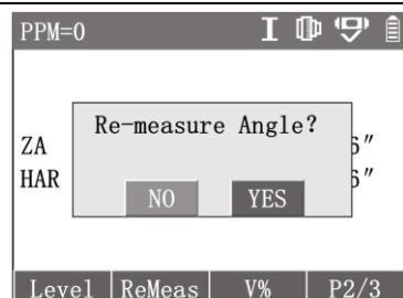
⑧Press [ESC] to exit {Re-measure} to the angle measurement.
