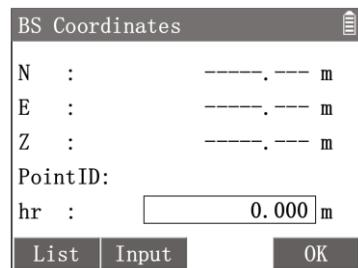
④ Aim at the backsight point and press [ENT] <YES> to set the orientation.
