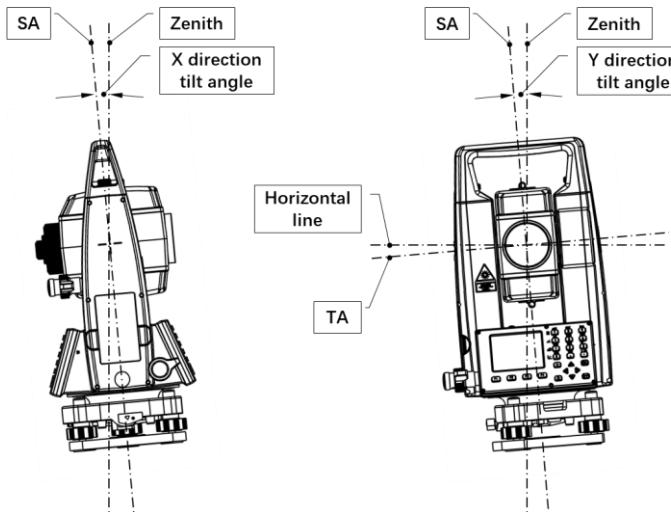
The SA tilt of the instrument is the angle between the direction of the SA and the direction of the zenith (plumb), which can be decomposed into two rectangular components, i.e., the X and Y direction tilt angle.
