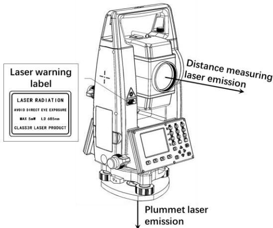
In accordance with the state of the international standard IEC 60825-1(2014-05), the product is classified as different Laser class on different working mode.
