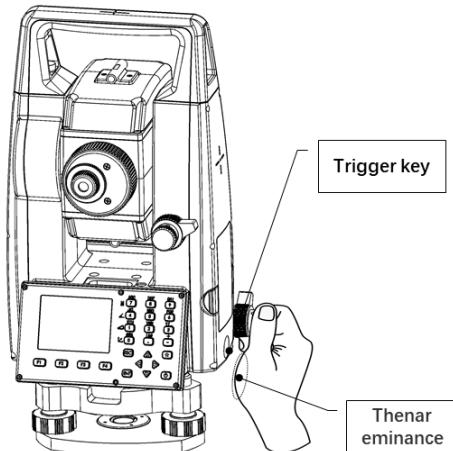
The trigger key is a special area on the side cover of the instrument near the horizontal drive. The trigger key is touch driven. It is designed to trigger the measurement function by lightly touching the area with the thenar eminence or any finger.
