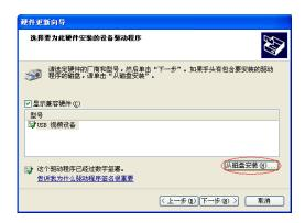
(6) In the following dialog box, click button of **<Browse (B)...>** once, select file "scicamd.inf" under the content where the drive is, and finally lick **<Determine>** once.
