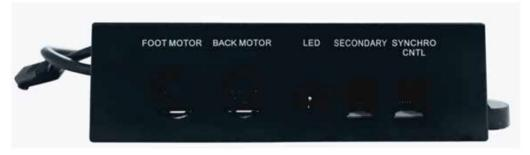
FOOT MOTOR : Foot lifting motor BACK MOTOR : BACK lifting motor
