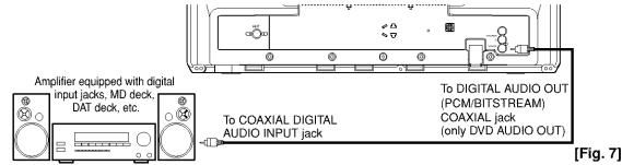
Using industry standard audio patch cords, connect one end to the Coaxial Digital Audio Out jack on the rear of the TV/DVD/VCR and the other to the Coaxial Digital Input on the audio system. Then select the Coaxial Digital Audio Input on the Audio System to listen to multichannel (5.1) DVD sound.
