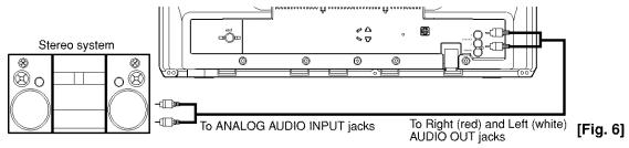
• Using industry standard audio patch cords, connect one end to the Audio Output Left (white) and Right (red) jacks on the rear of the TV/DVD/VCR, and the other end to the audio input Left (white) and Right (red) on the audio system.
