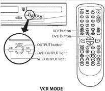
Press [VCR 👓 ] on the remote control. (The VCR OUTPUT light illuminates.)
