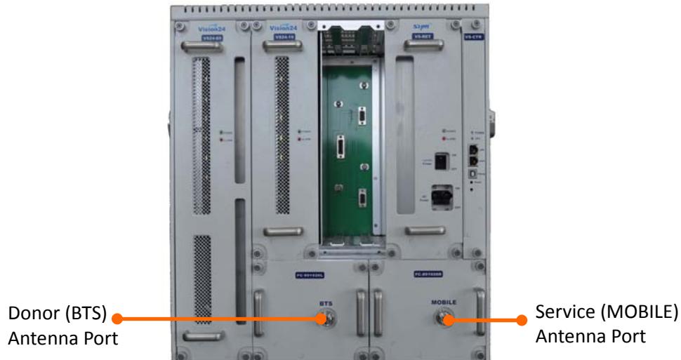
[Figure 2-6] Antenna port on the Vision
