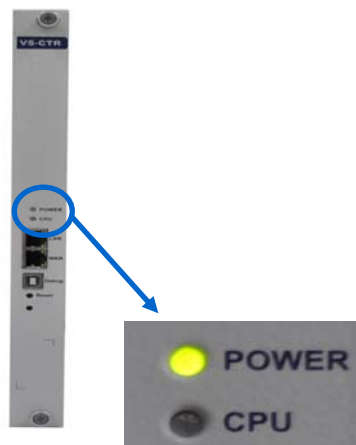
[Figure 3-2] Controller Front Panel Controls and Indicators
