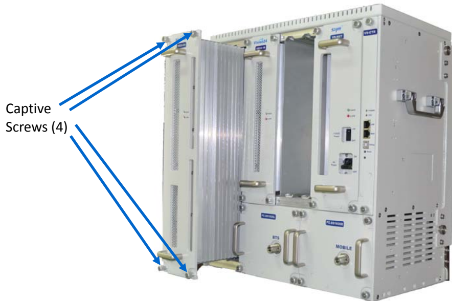
[Figure 4-1] 800/900 MHz Service Card Replacement
