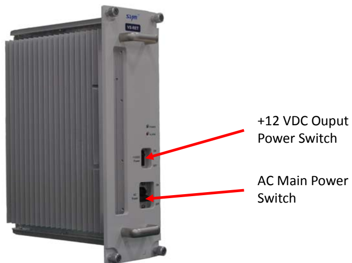
[Figure 1-7] Rectifier view
