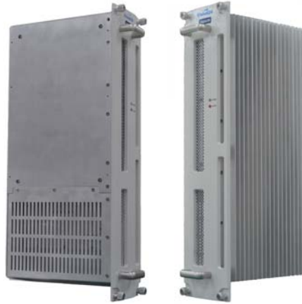
[Figure 1-5] 800/900 MHz Service Card view
