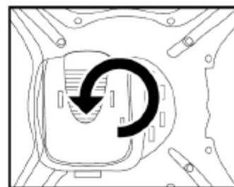
**2.Aiming the camera at the interface on the main body and rotating the camera in anti-clockwise direction to make it screwed.**
