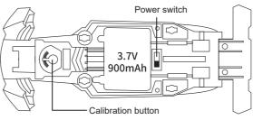
Calibration button: Adjust the lever on the bottom of the vehicle until the vehicle travels in a straight line
