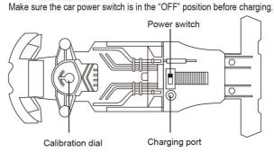
Calibration dial: Adjust the lever on the bottom of the vehicle until the vehicle travels in a straight line
