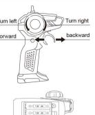
Pairing: Switch on the remote control, and then press the on/off switch on the vehicle Wait until the LED indicator on the remote control stops flashing and stavs constant. his indicates that pairing was successful.
