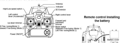
Open the back cover at the back of the transmitter. Load 4PCS "AA" alkaline batteries correctly into the battery compartment as per the correct polarity shown on the battery compartment.
