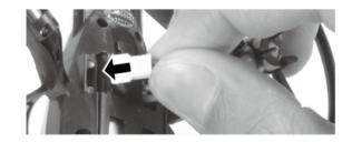
Step 2: Insert the power line into the quad copter and place it on the level ground.
