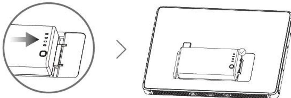
Note: Ensure to press the Battery Remove Button before remove the battery.
