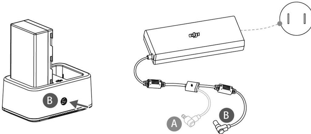
Tips: The charging hub can charge two batteries at the same time. It will take a longer time to charge the Intelligent Flight Battery and remote controller together.
