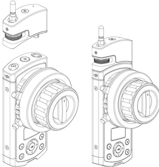
3. When used with the Ronin-MX, connect the Communication Port on the Motor to the LB Port and the P-TAP Port by using the provided Power and Communication Cable.
