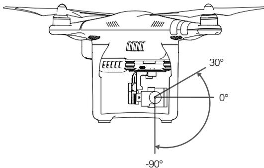
Use the gimbal dial on the remote controller to control the tilt movement of the camera.
