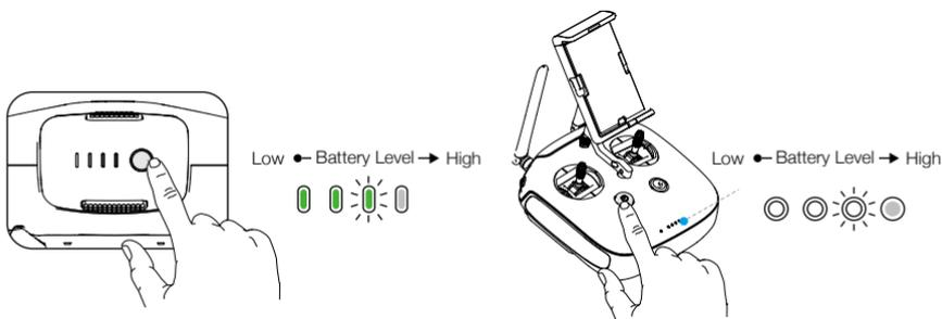
Press once to check the battery level. Press once, then again and hold to turn on/off.
