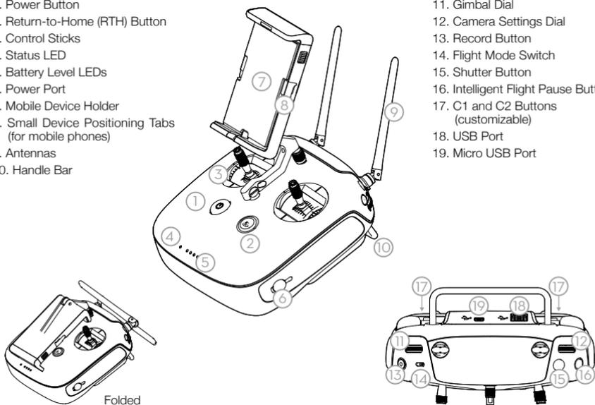
The default flight control is known as Mode 2. The left stick controls the aircraft's altitude and heading, while the right stick controls its forward, backward, left and right movements. The gimbal dial controls the camera's tilt.
