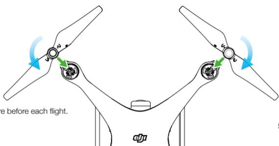
⚠ • Check that the propellers are secure before each flight.
