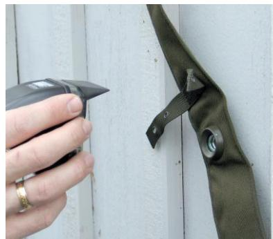
12. The SES is generating a "primary room" audio cue. Put one RAD installed in primary room in front of the laser detectors. Repeat the procedure when SES is generating a "secondary room" audio cue. The SES will confirm each Room ID.
