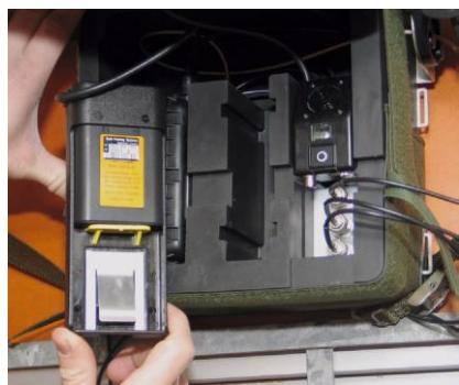
10a. Install **Rechargeable battery**. Remove the Battery Unit (BU) and insert the battery. Verify that "Tampering kill" is heard from the speaker.
