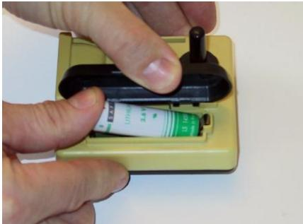
2. Take the SID and check if the battery is installed. Make sure to use Lithium battery 3.6V 2.25 AH LI AA.
