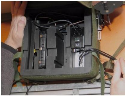
8. Open the SES flap and connect the detector/reflector belts into the SES.
