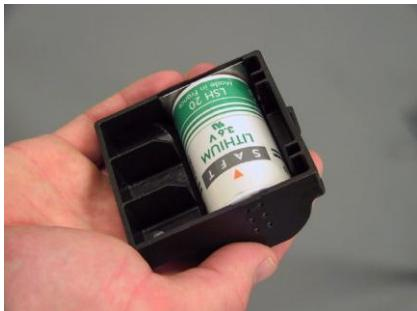
10c. Put the battery in the battery holder. Verify that "Tampering kill" is heard from the speaker.
