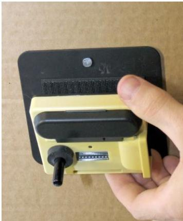
4. Install the SID according to information displayed on the SID (S=structure ID and r=room ID).
