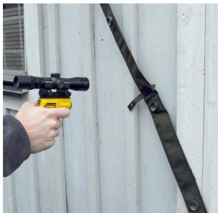
11. Use the CGUN and shoot a RESET Command. Message "RESET WALL TYPE NO" is heard from the speaker. The speaker confirm that wall type level in primary room is set to default value given by the SID. To start the configuration of the RADs, shoot an ACCESS Command with the CGUN.
