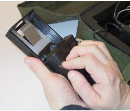
10b. Install **Non-rechargeable battery**. Remove the BU. Remove the battery holder from the BU.
