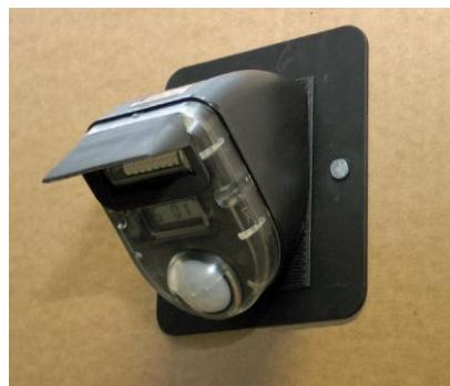
5. Install the RADs according to information displayed on the RAD (S=structure and r=room ID).
