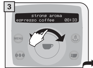
3 Select the desired beverages by navigating the click wheel with your finger.
