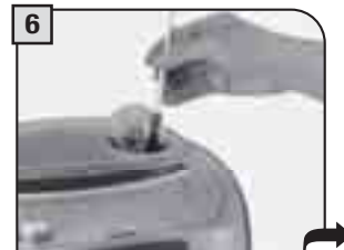
6 With the brush, clean the pre-ground coffee compartment.
